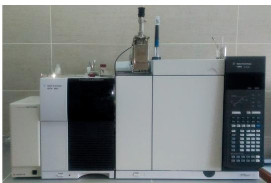
Fig. 1. A pyrolytic system for investigation of geological objects
